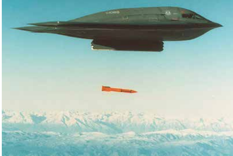
▲ A B-2 Spirit stealth bomber drops a mock-B61 gravity bomb. The B61 is a Los Alamos–designed weapon that's currently undergoing a life extension program. Photo: U.S. Air Force
